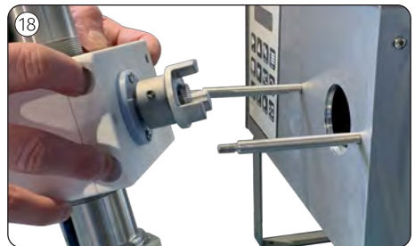
Remember to check that the clutch teeth fit, otherwise the pump housing cannot be put back on completely.
