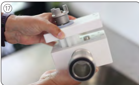
Put the pump housing together again.
